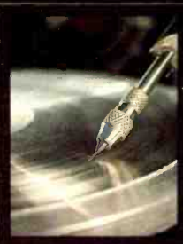
V-groove Lapidary Final polishing of stylus, mounted on beryllium shank.
