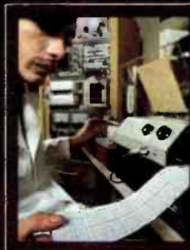
Graphic Recorder Plotting of individual 530-mp frequency response.
